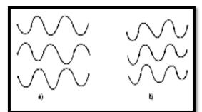
If the phase difference is  $180^{\circ}$  then the two waves are said to be in antiphase and if it is  $0^{\circ}$ , then they are in phase
